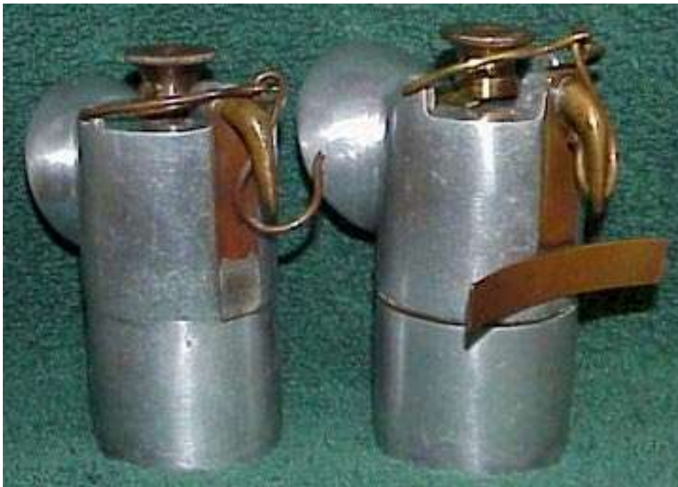
(left) Back view shows "Bull's Horn hook which screws into threaded casting.
